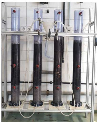
Fig. 1. Experimental setup for the column tests in the laboratory
